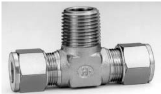
PM8TTM6BR COMPRESSION X ½ COMPRESSION X 3/8 MALE NPT, TEE
